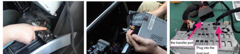
Complete the transfer of air conditioning panel
